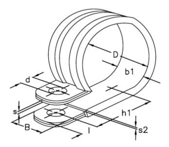
$\begin{array}{lll} b1 & = 18.5 \\ d & = 6.4 \\ Diameter D = 25 \\ h1 & = 23.7 \\ I & = 6.0 \\ s & = 0.80 \\ s2 & = 1.5 \\ Width B & = 15 \\ \end{array}$
